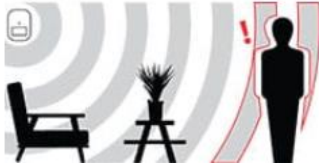
Figure 14: The detection of PIR sensors
