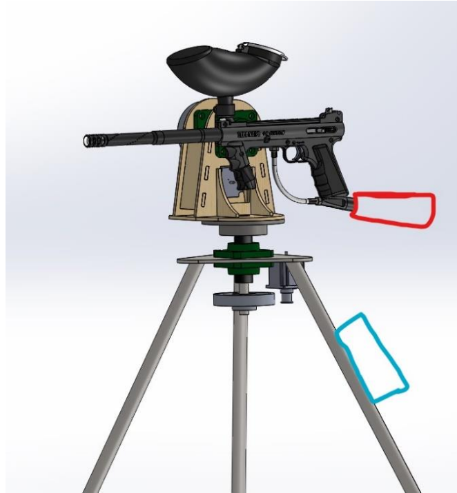
Figure 56: Mount for compressed air tank
